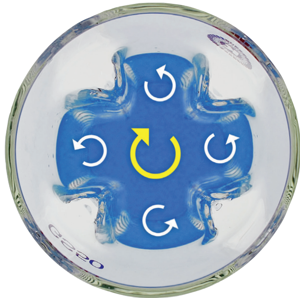
GS vessel principle (viewed from top)
